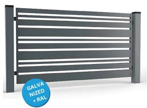
The Diverso System is a fence that combines metal profiles of 30x20, 60x20, 80x20, and 120x20, arranged alternately. The gap between the profiles is only about 20-30 mm. The welds are cleverly concealed within the slide guide rail section!
